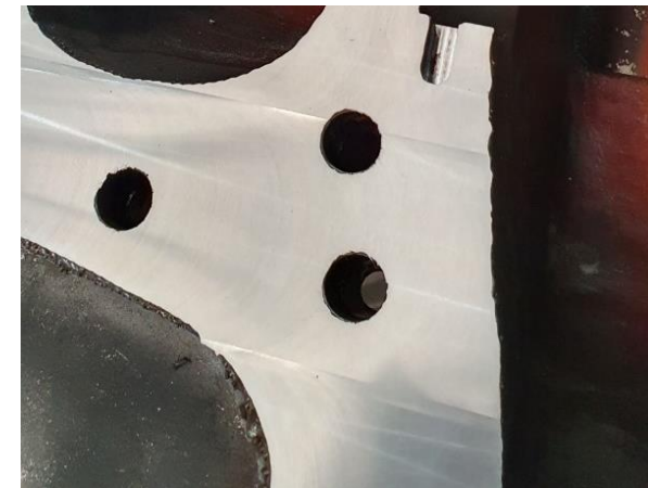
After LaserBond reclamation process
