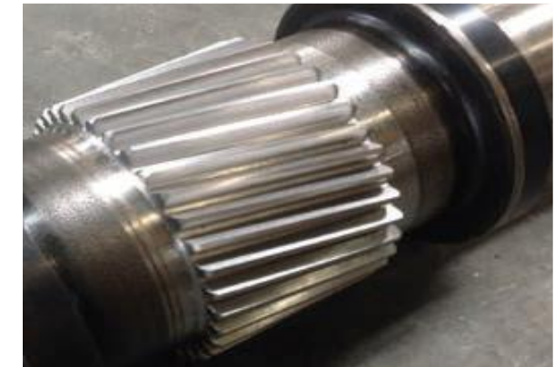
After LaserBond reclamation process
