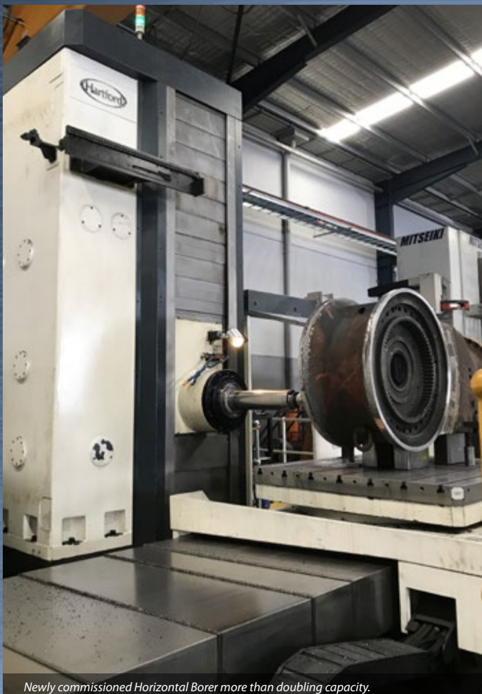
Newly commissioned Horizontal Borer more than doubling capacity.
