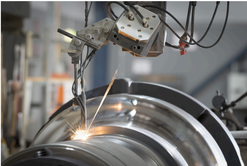
Laser cladding is a high-performance additive manufacturing procedure, which utilises precisely controlled energy from a high power laser to metallurgically-bond a surfacing material to a substrate to provide very high performance surfaces to new parts for extended operating life. With this precise control, a welded or metallurgical bond is achieved with minimal effects of heat on both the substrate and surface material.
