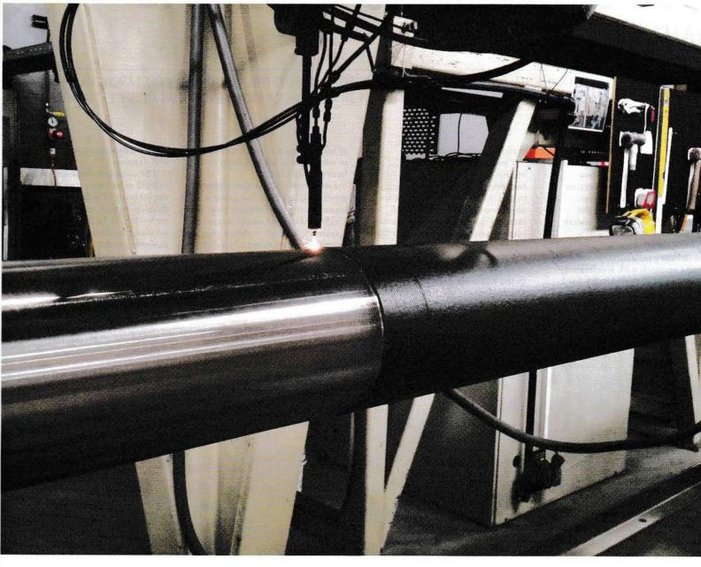
developed a new laser deposition method, which virtually eliminates substrate dilution and detrimental heat effects. This technology makes laser cladding technology available and economic to a wide range of industrial applications, in particular, high wear applications common in resource industries, and as a replacement for hard-chrome, as used on hydraulic cylinders in mining and drilling.
