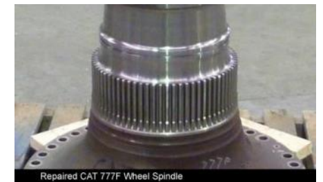
Repaired splines and bearing surfaces
