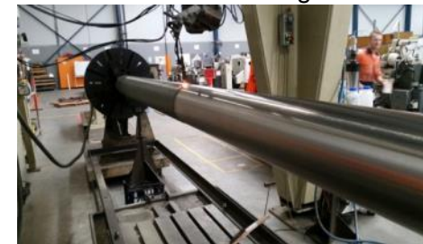
LaserBond® cladding 8m ram
