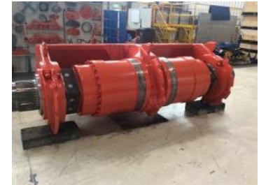
Reman of UG cutter drum assembly
