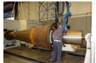
Crusher shaft repair
