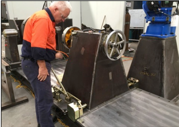
Pre Delivery Commissioning - Testing the heavy-duty tailstock carriage mechanism developed by LaserBond.
