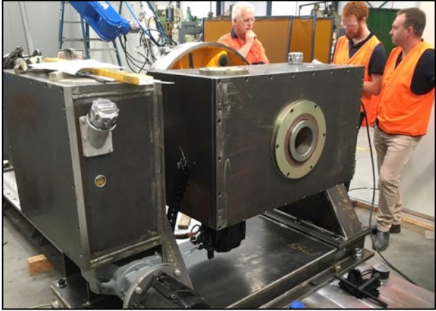
Pre Delivery Commissioning – Reviewing accuracy of movement available with the LaserBond 2-axis heavy component manipulator.
