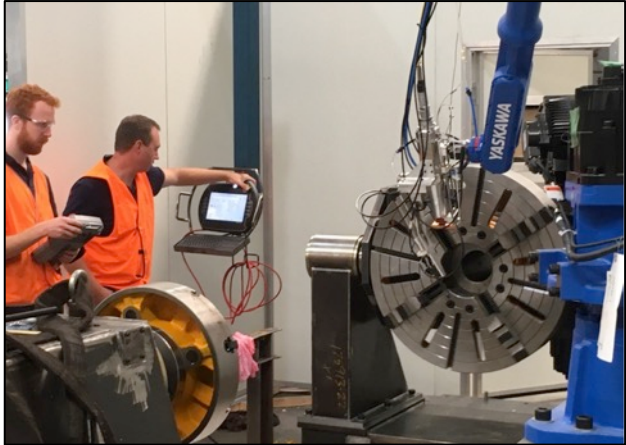
Pre Delivery Commissioning – Testing operation of 6-axis robot and 2-axis work piece manipulator.
