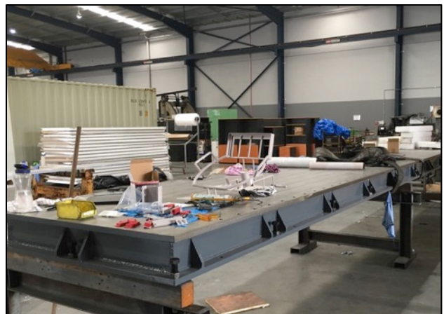
Pre Shipping Inspection – 8m heavy-duty base frame that supports manipulator and work piece.
