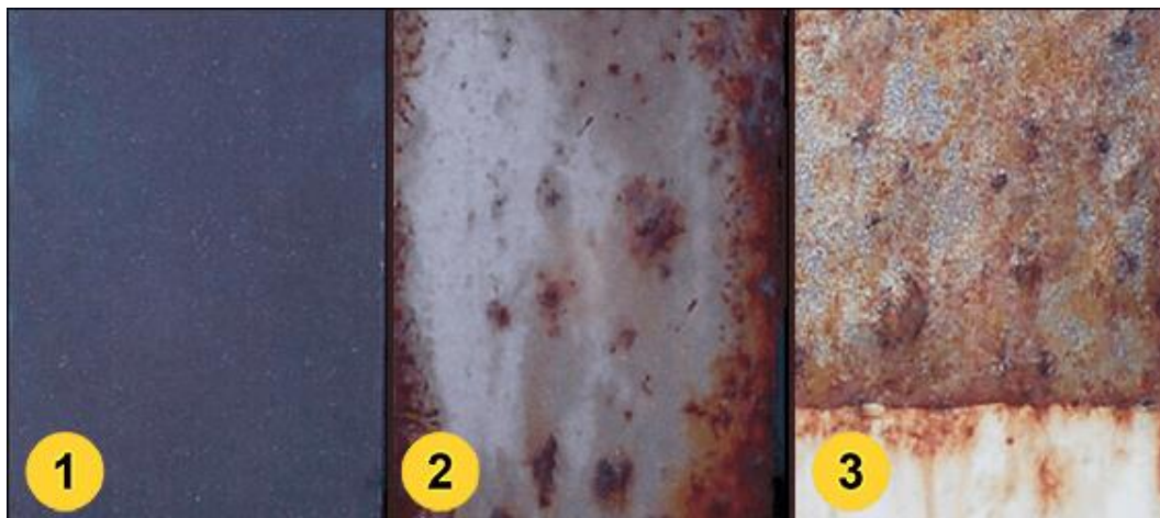
Figure 12: 1) HVOF, 2) Tibaloy 400 & 3) Hard Chrome. Coated Steel plates after 18 months of atmospheric exposure and weekly spraying with salt water. 21
