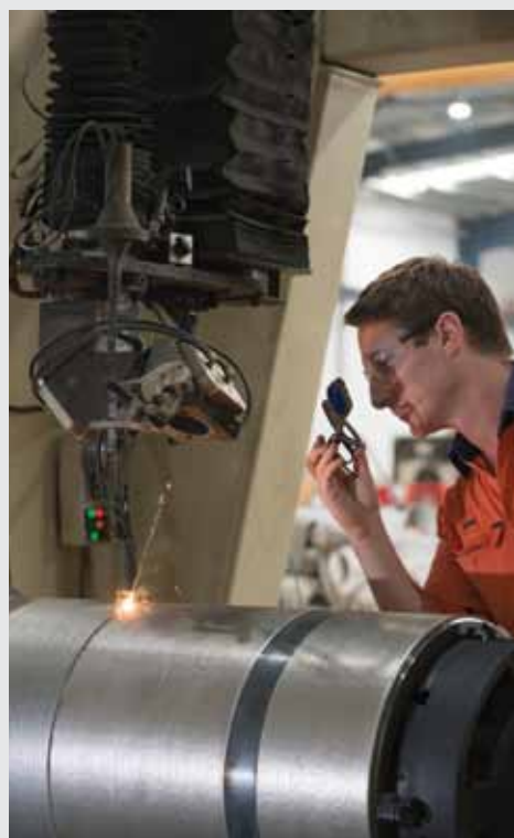
Temperature sensitive components are repaired with minimal risk using Laserbond's deposition process.
