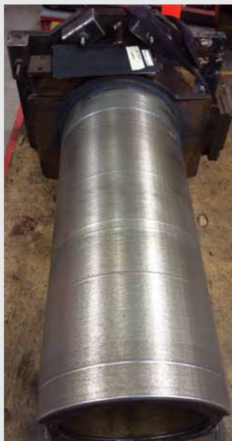
Underground mining road header boom after laser treatment.
