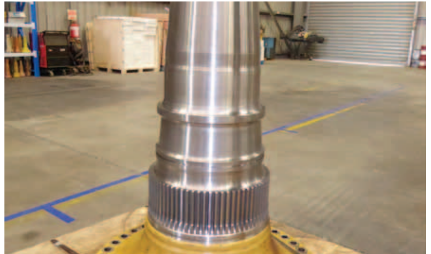
The CAT 777F dump truck spindle ready for shipping back to customer.
