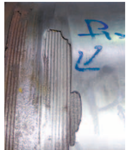
((left) Wheel spindle bearing journal fretting and spline damage before LaserBond repair. (right) Delamination of previous spray repair.
