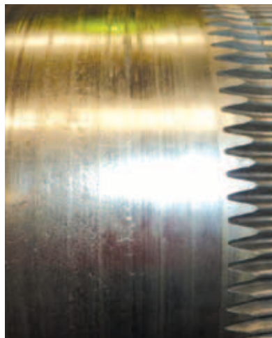
((left) Wheel spindle bearing journal fretting and spline damage before LaserBond repair. (right) Delamination of previous spray repair.
