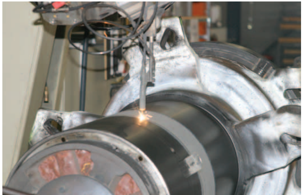
LaserBond cladding process of mining drum to restore working surface to OEM specifications.
