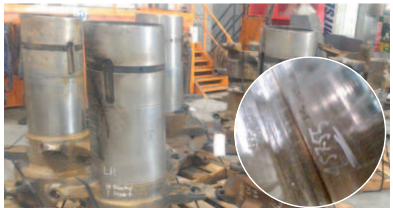
Disassembled worn and damaged drum components in receiving area. Inset: Galling of steel on steel seizure.
