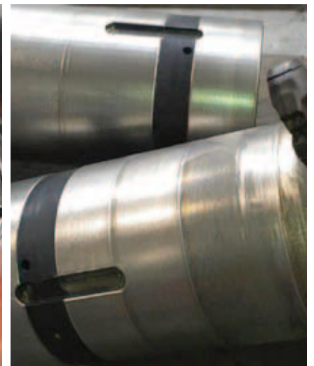
Repaired and refurbished inner and out drum components, with improved metallurgy to prevent galling.
